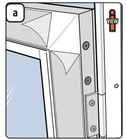
Starting at the mitered corners, remove the clear protective tape from both the interior and exterior of door frame, if applicable.
