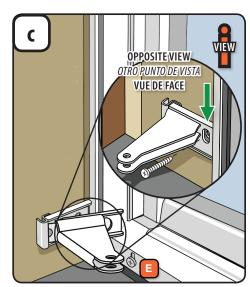
1. Attach the arm from the installation kit to the base by inserting the tabs on the arm into the slots in the base. Fasten with a 2" screw from the installatio kit.
