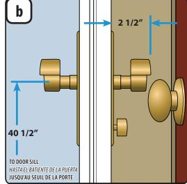
Most homeowners prefer to have the storm door handle on the same side as the entry door handle. In shallow door openings, this can cause the two handles to interfere. Check for potential interference using the rough measurements. If you anticipate that there will be interference, purchase a storm door that is hinged on the opposite side of your entry door. See page 2, Figure 3 for detailed hardware depth requirements.
