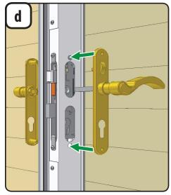
With handle levers held horizontal, install both handle assemblies onto door. Spindle will pass through square hole in lock case and into other handle. Attach trim plates together using two 1 1/2" pan head screws.
