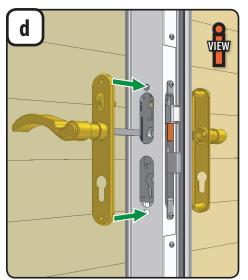
1. With handle levers held horizontal, install both handle assemblies onto door. Spindle will pass through square hole in lock case and into other handle. Attach trim plates together using two 1 1/2" pan head screws.
