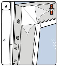
If applicable, start at the mitered corners and remove the clear protective tape from both the interior and exterior of door frame.
