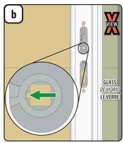
Look into handle holes on door to make sure lock case is oriented properly. Notch in square spindle hole should be facing away from glass panel.
