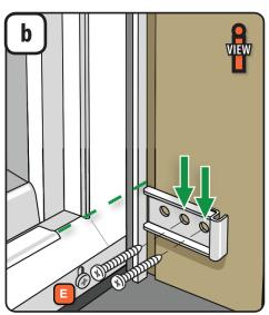
Position base from installation kit onto door jamb by touching front of base to back of hinge rail (or as close as possible), and align top of base with top of retainer channel.
