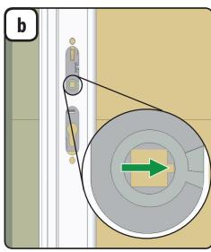
Look into handle holes on door to make sure lock case is oriented properly. Notch in square spindle hole should be facing away from glass panel.
