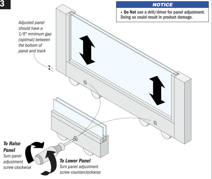
Raise the side(s) of the panel to be adjusted. Insert a phillips screwdriver into the roller socket(s) and adjust lead panel for an equal gap between the panel and side jamb. Close and lock door. Engage interlock weatherstrip between the lead panel and the next panel and adjust as needed. Repeat for all subsequent panels.
