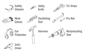
Tools needed for unit removal may vary due to existing construction, unit type, fasteners, and interior or exterior removal method. Additional tools may be required.
