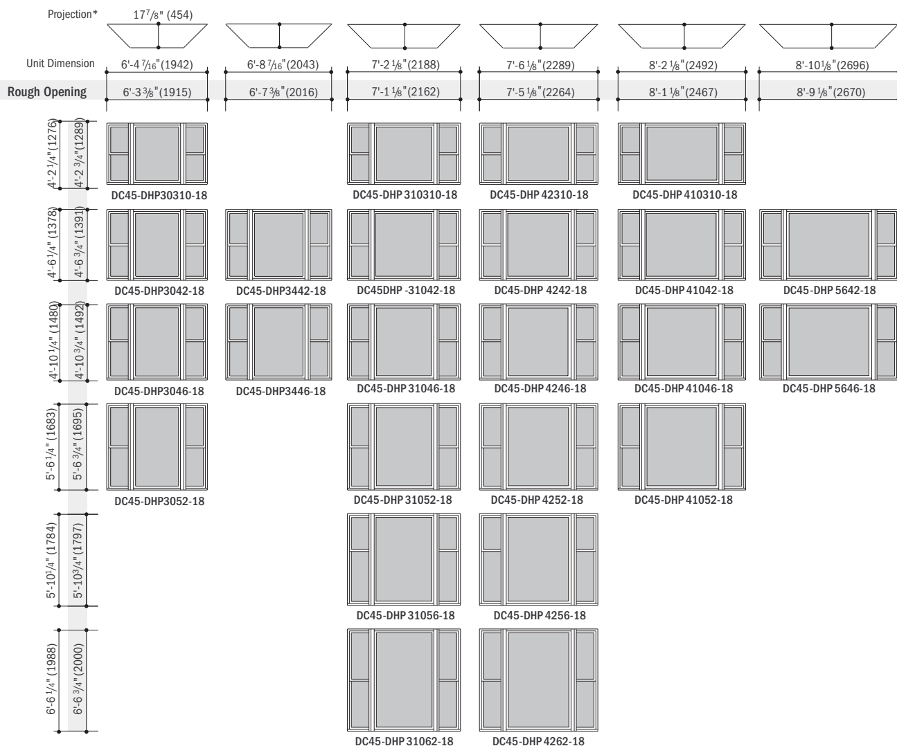
Tilt-Wash (DC) and Tilt-Wash II (TW) 45° Angle Bay Window Standard Unit Sizes
