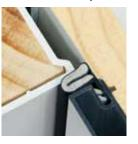
Durable rubberized Santoprene® gasket-type weatherstrip is applied to the frame (sides and head jamb) and engages when the door panel is closed. The panel has a sweep system at the sill that completes the perimeter protection.
