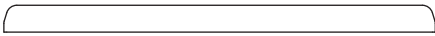
A 2 1/4" (57) width grille is available for most units to simulate a meeting rail or a multi-unit combination such as a transom over a window or patio door.
