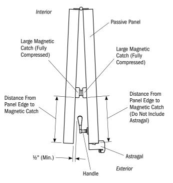
Passive Panel - Handle Clearance Top View
